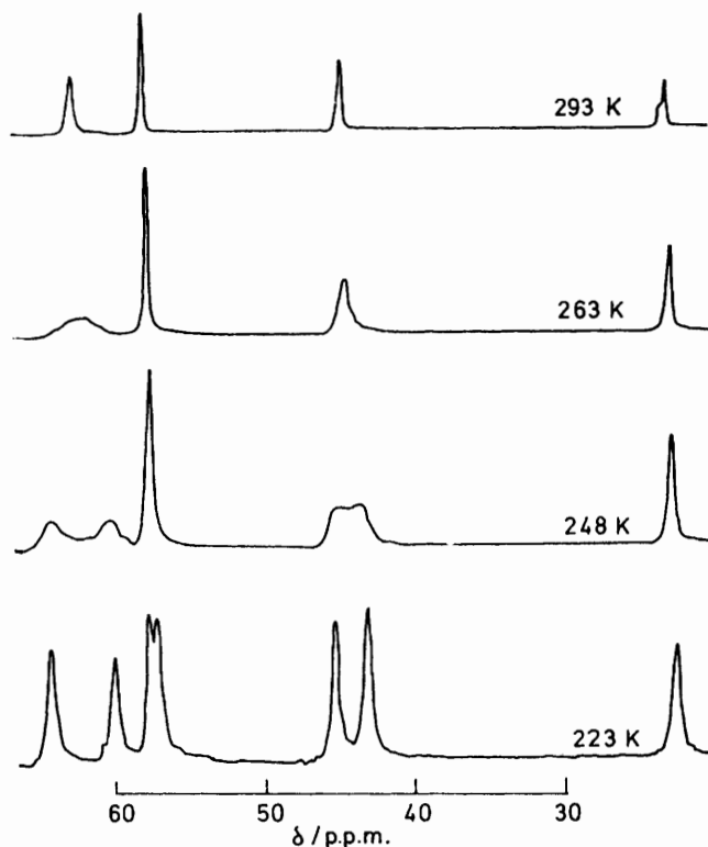
FIGURE 6 Variable-temperature ^{13}\text{C} n.m.r. spectra of [\text{Cd}(\text{L}_b)]\text{[NO}_3\text{]}_2 in [\text{}^2\text{H}_3\text{]}_{\text{nitromethane}} (chemical shifts relative to internal dioxan, \delta = 67.3 p.p.m.)
